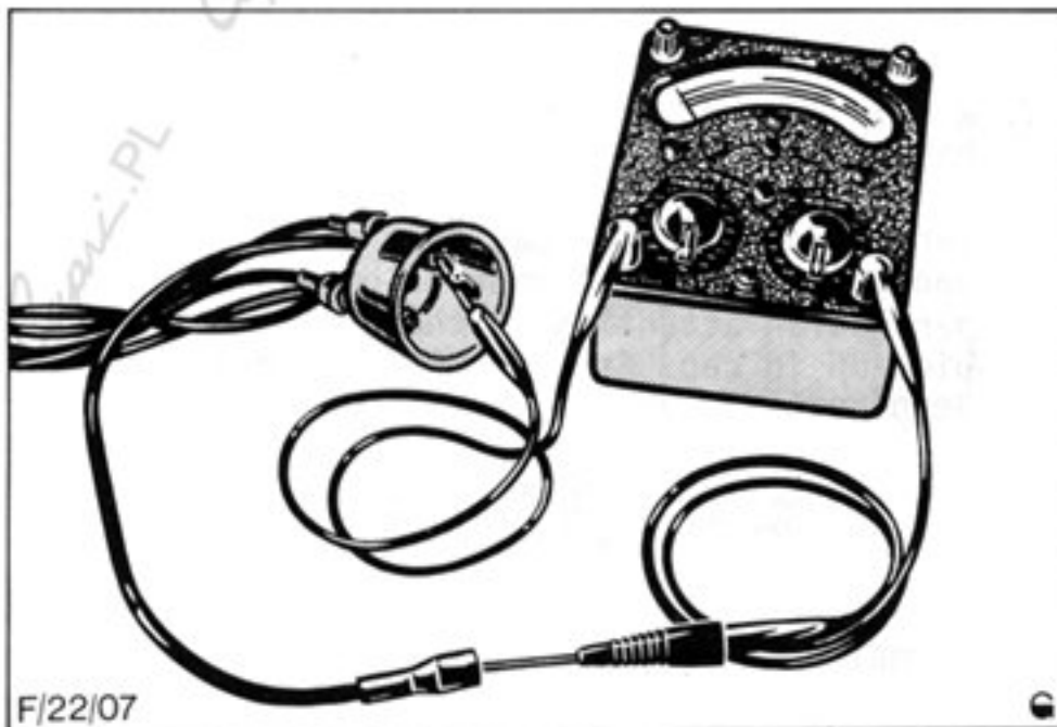
Fig.28. HT lead resistance being checked. (Ohm meter shown).
