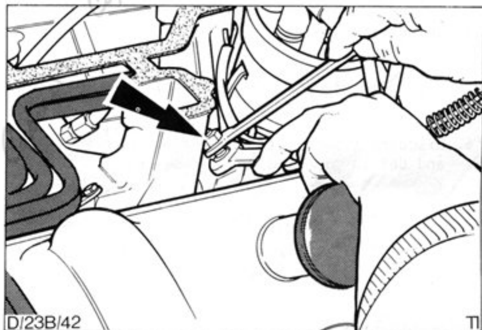
Fig.93. Injector supply pipe removal.
