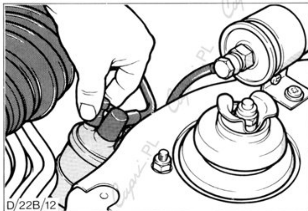
Fig.54. LT lead removal from coil pulling terminal NOT lead.
